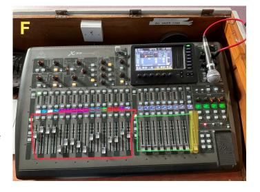
3. Each of the 16 channels has a fader (slider) to control the volume of each instrument or voice. Above each fader you will see an illuminated box which tells you what is controlled by that fader. Moving a fader up will increase the volume of that instrument or voice. See picture G.
